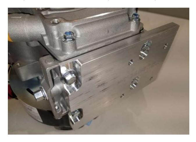
4. Align the OEM engine plate from the original engine to the aluminum plate's tapped holes. The exhaust hole in the OEM plate should be towards the front of the engine.
